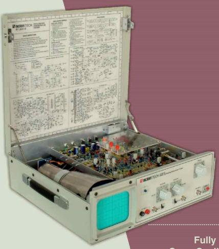
Scientech Oscilloscope Demonstrator Trainer ST 2001E is specifically designed for the study of working of an oscilloscope in an open form.
